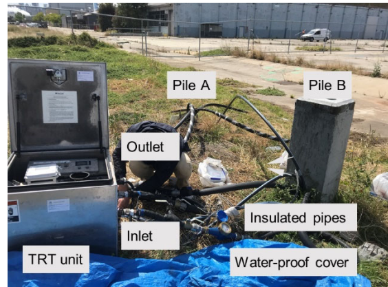
Figure 3. In-situ TRTs set up
