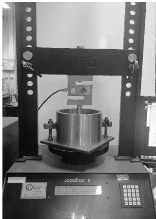
Figure 3. Modified oedometer test setup
