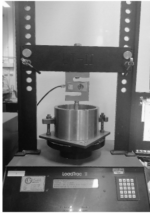
Figure 3. Modified oedometer test setup
