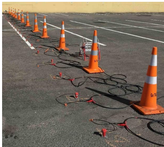
Figure 1: An example of a 4.5-Hz seismic refraction geophone used to record ambient noise.
