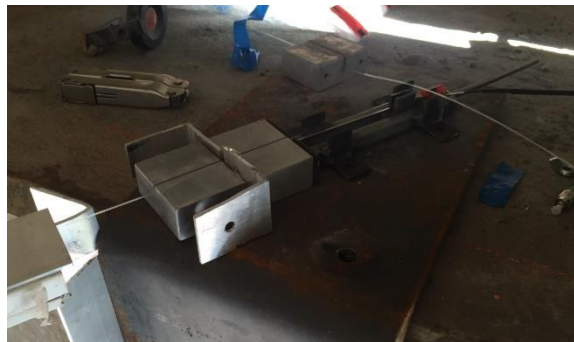
Figure 8: Sensor Cable in Clamping System with Tensioning Tool
