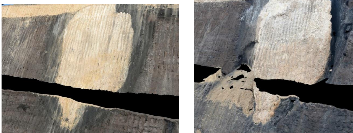
Figure 5: Before and after models of batter deformation
