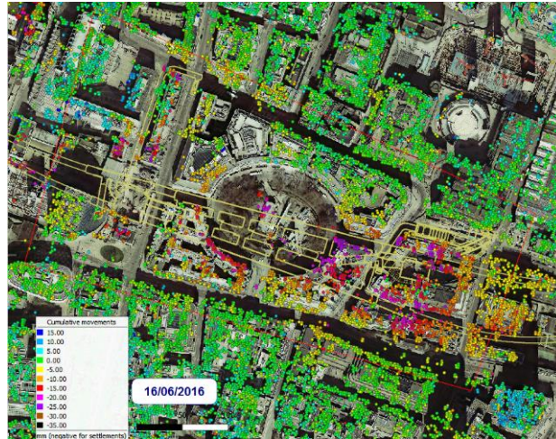
Figure 7. Recorded settlement at Finsbury Circus after almost 4 years of work
