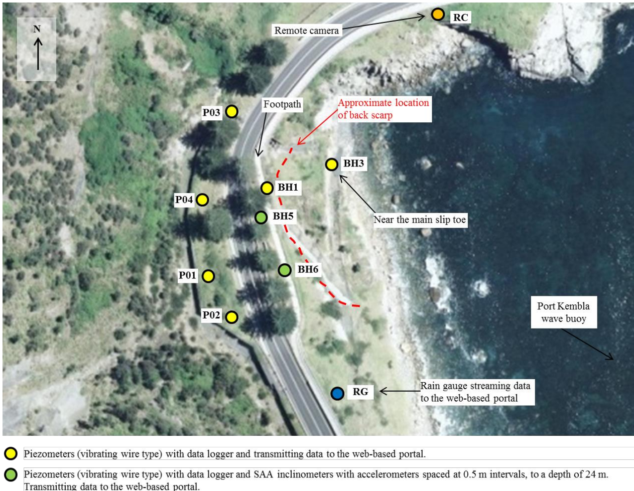
Figure 4: Borehole locations and Instrumentation plan.
