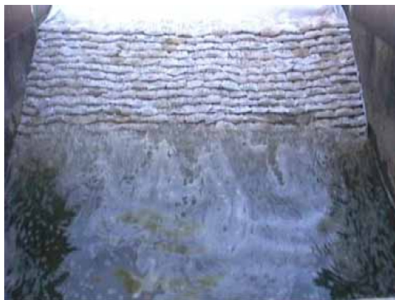
Figure 5. Model during wave attack ( H_s \sim 1.4\text{m} )
