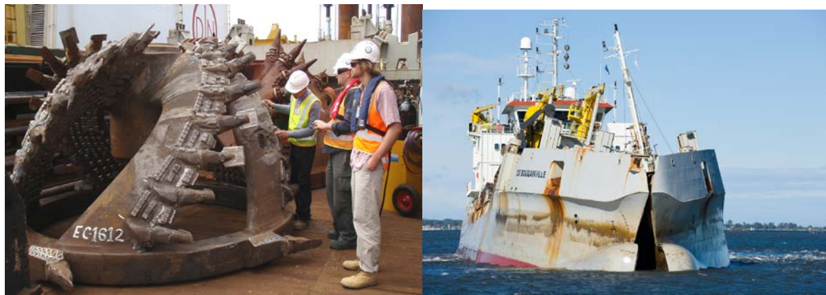
Figure 3: Cutting Head from Cutter Section Dredge and Split Hopper Dredge – De Bougainville
