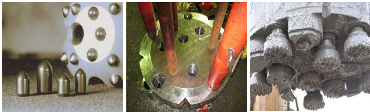
Figure 7: typical drill bits and button inserts (left) for DTH hammers, assembly of individual DTH hammers and base plate of cluster barrel (centre), individual drill bits of a cluster barrel (right).
