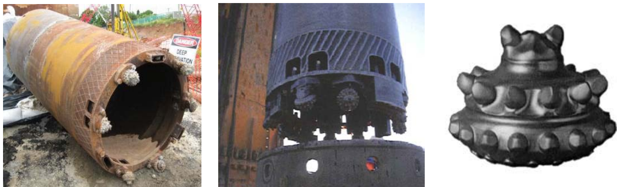
Figure 3: Typical air roller core barrel (left & centre) and single roller cone drill bit (right).
