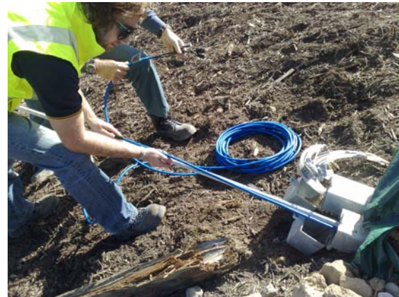
Figure 13: Thermistor insertion for reading (blue on left) and O 2 tube outlets (right).
