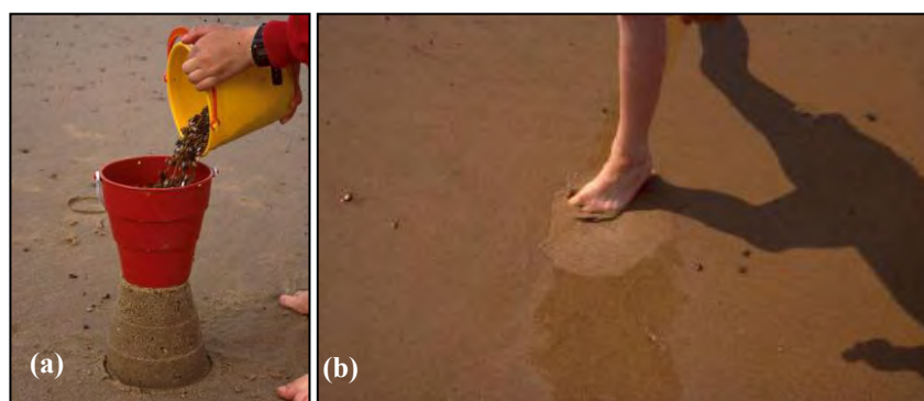
Figure 1: (a) Unconfined compression of sand. (b) Undrained shearing of dense sand (after Atkinson, 2008).
