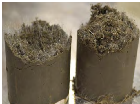
Figure 6: A typical fibre reinforced cement-treated clay sample
