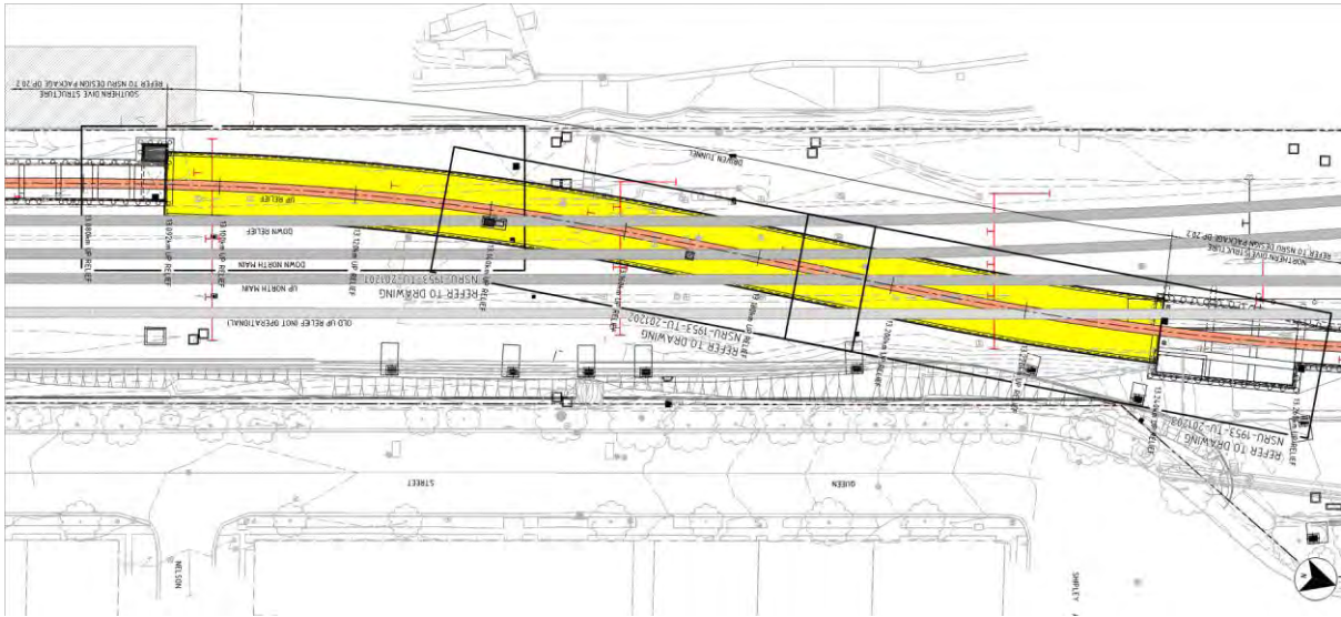
Figure 1: Tunnel plan alignment.
