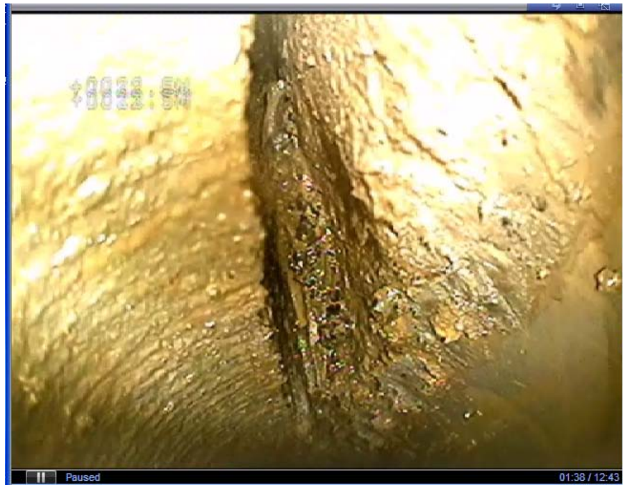
Figure 5: Vertical fracture in borehole beneath viaduct location
