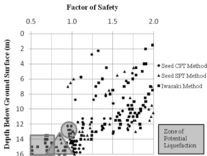
Figure 8: Iwasaki method compared with Seed methods for M=6.3
