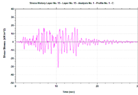
Figure 7: Shear stress time history on the SAND1 layer. Figure 8: Stress time history at SAND2 layer.
