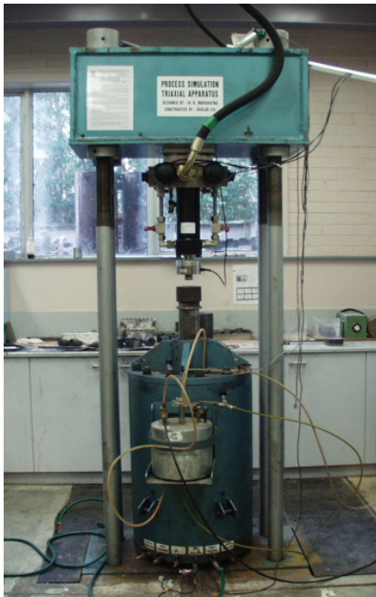
Figure 1: Cylindrical triaxial apparatus equipped with a dynamic actuator at University of Wollongong Figure 2: Normalised shear strength for latite basalt aggregates (after Indraratna et al. , 1998)
