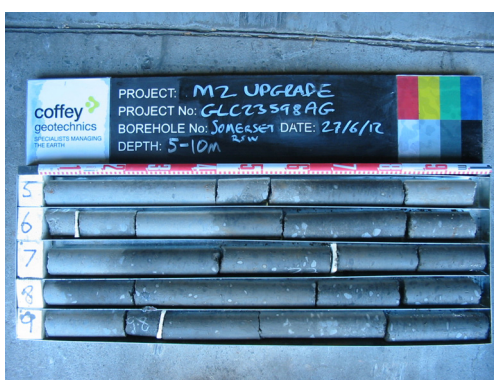
Figure 10: Core samples of the stabilised DGB20.
