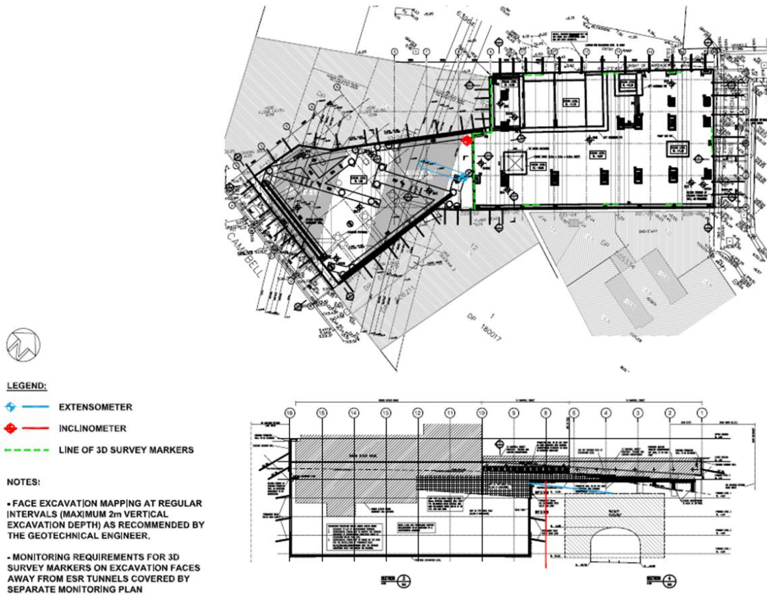
Figure 13: Plan and Section Closes to ESR Tunnel (4 – 10 Campbell Street, Sydney)
