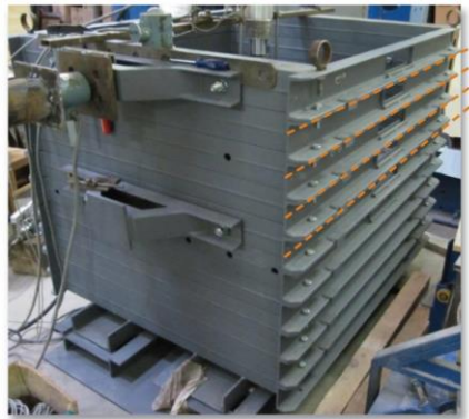
Figure 2: Multi-layer shear box to investigate stabilization effect at various levels above geogrid
