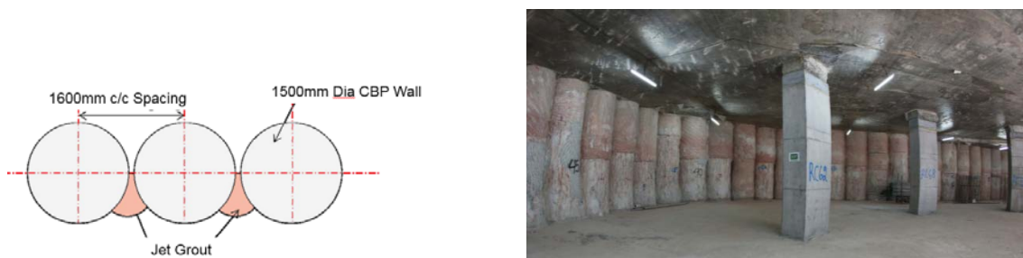
Figure 3: Proposed Contiguous Bored Pile (CBP) Wall
