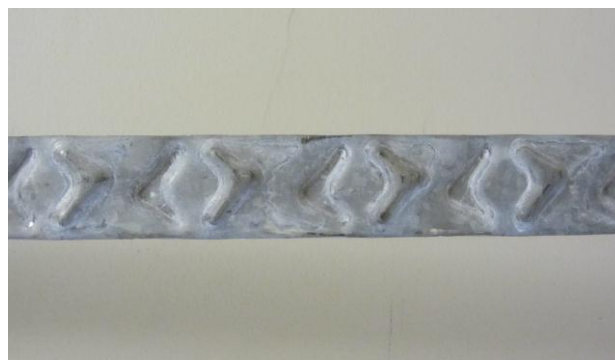
Figure 2: Photograph of indented steel strip
