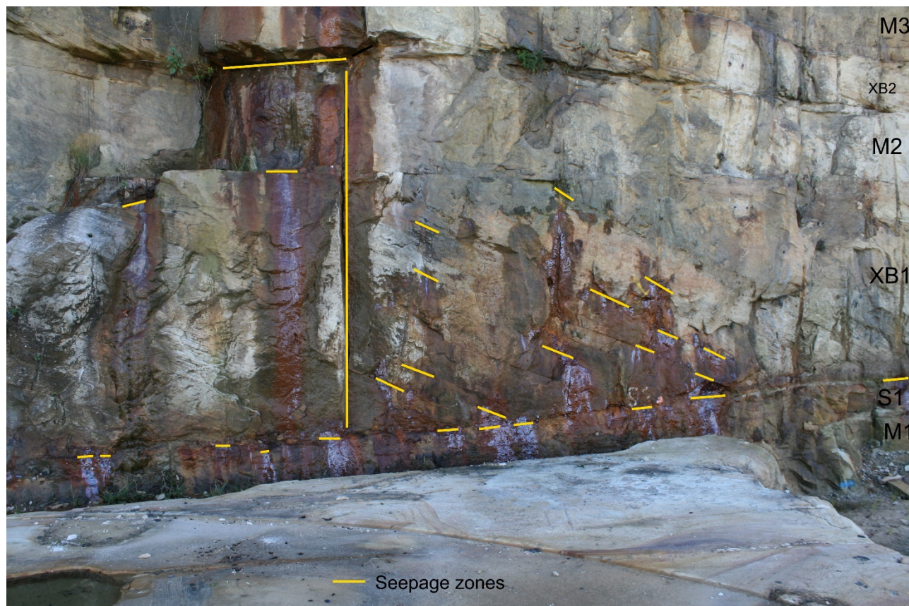
Figure 8 Hydrocarbon impacted seepage visible on bedding planes at Ballast Point, Birchgrove. Several zones of groundwater were encountered in the Hawkesbury Sandstone at Mortlake (Figures 1, 4 & 9). The perched zone identified localised seepage water present at the fill / sandstone interface, and was influenced by fresh surface infiltration. The upper groundwater zone was present within a water bearing zone highly weathered, iron stained sandstone present beneath the site (depicted in Figure 4), at an approximate depth of 6 – 8m below the surface. Below this cross bedded and laminated (with siltstone) sandstone, massive fresher sandstone was encountered which was saturated (the lower groundwater zone) and continually seeped into the excavation. The base of upper groundwater zone overlying the fresher massive rock an erosional surface characterised by a siltstone breccia.
