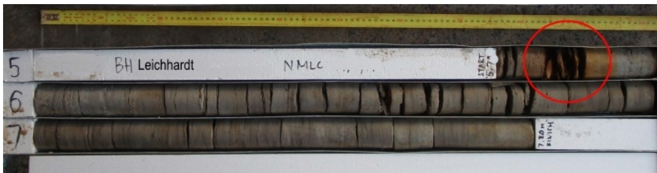
Figure 7 Migration pathway for chlorinated solvents along major bedding plane, Leichhardt
