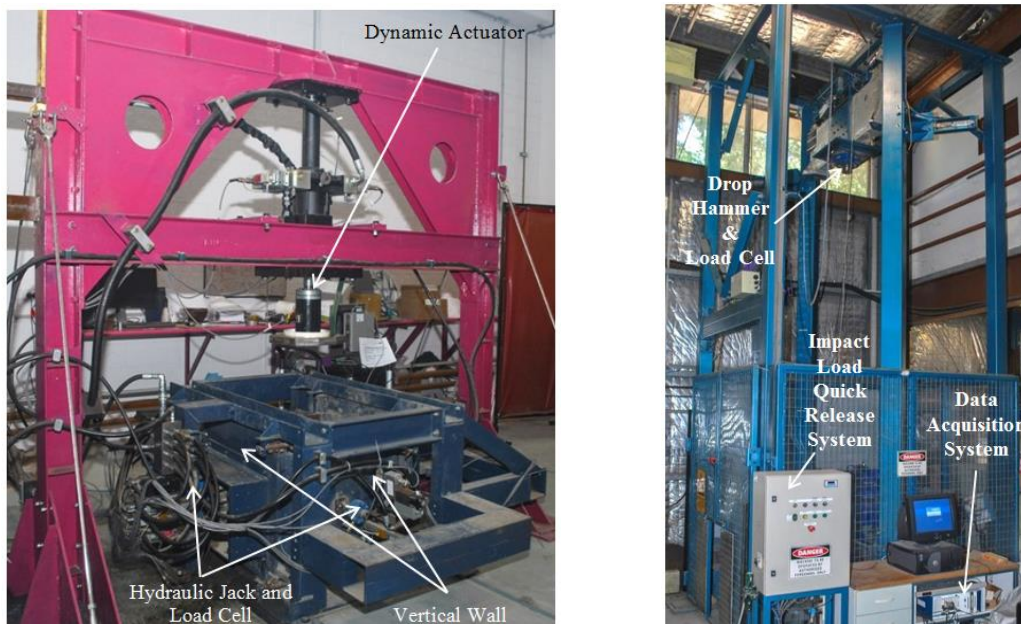
Figure 29: (a) Process Simulation Test Apparatus; (b) High Capacity Drop Weight Impact Machine
