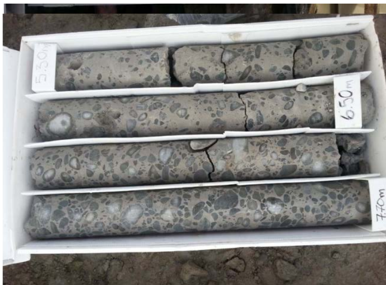
Figure 5. Quality control coring of DSM columns showing varying gravel sizes from different layers mixed through the column profile.
