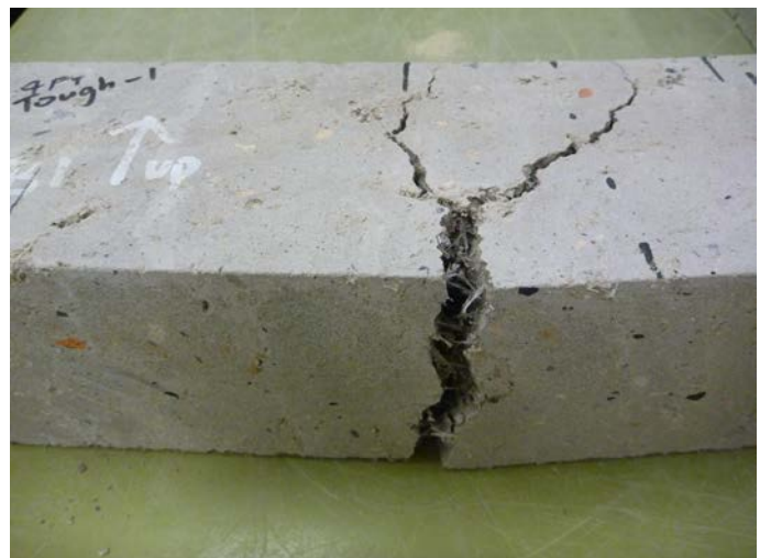
Figure 3: Typical crack pattern in a sample subjected to 4-point bending
