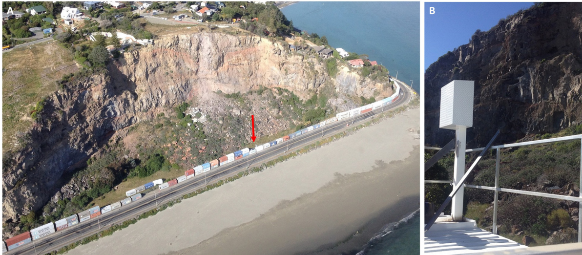
Figure 4. Laser scan monitoring Shag Rock Reserve, Sumner; A, aerial of Shag Rock Reserve cliff face and reserve area, the monitoring container location is shown with the red arrow; B, laser scan unit in monitoring box mounted in the monitoring container (as indicated by red arrow in photograph A).
