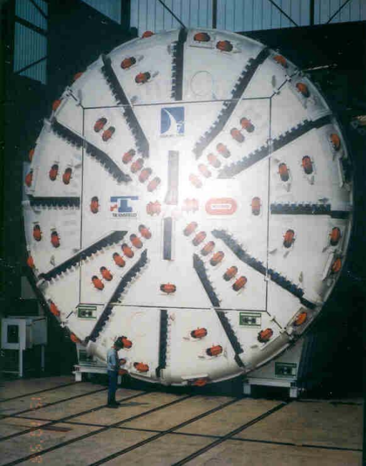
Slurry TBM Head
